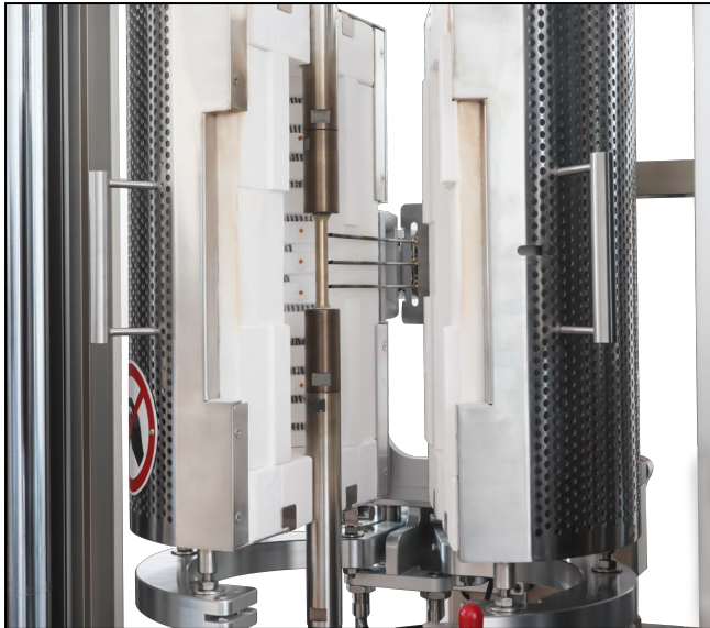
Open high-temperature furnace
